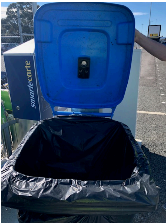
Figure 17 Car parking bin with sensor
