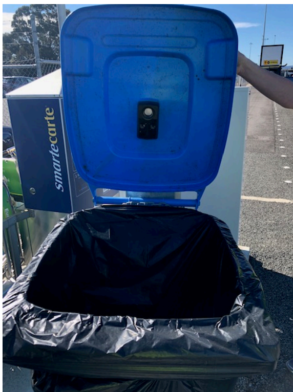
Figure 13 Car parking bin with sensor
